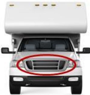
Air-intake grilles for vehicles
